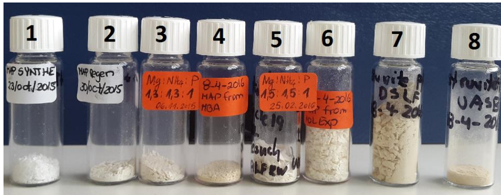
Figure 31. Struvite and recycled solids obtained from synthetic WW and the different enriched reclaimed solutions. Numbers correspond to the order in table 10.
