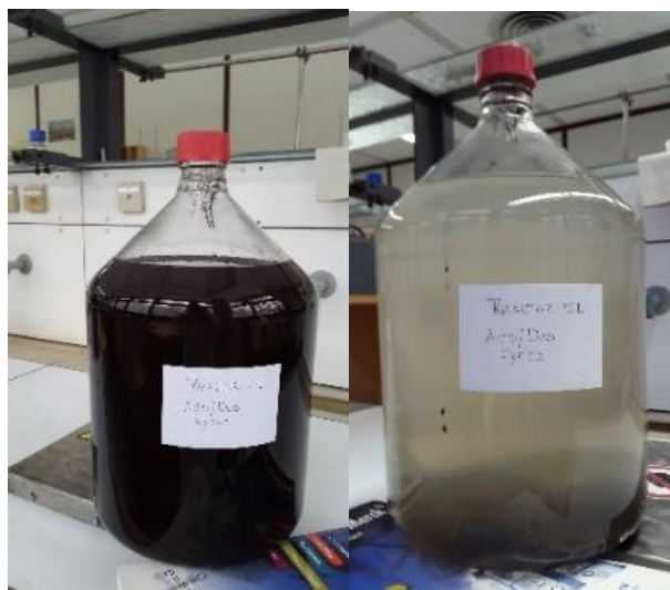
Figure 15. Separation of the magnetic particles before and after using a strong hand magnet.
