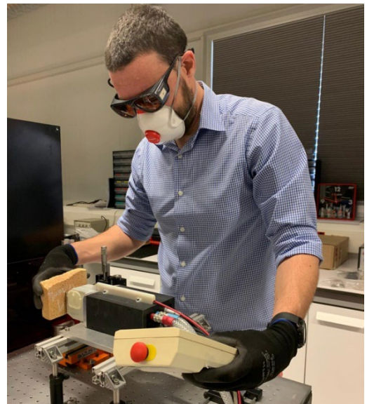
Figure1. LIBS sensor operating at the UMALASERLAB facilities on the analysis of a refractory material.
