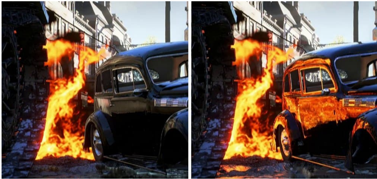
Figure 2.5: A scene rendered using Rasterization (left) versus a scene rendered using ray tracing (right) [5]
