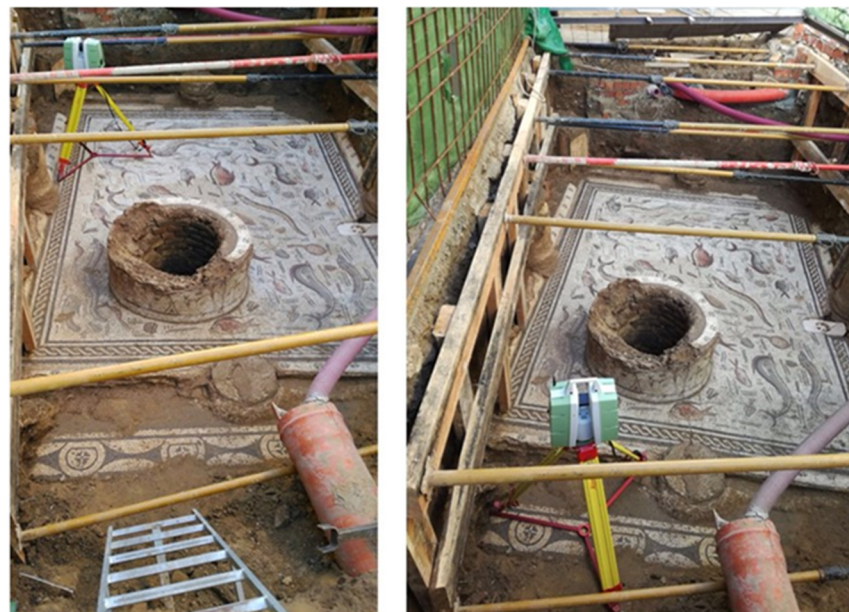
Figure 8. Data acquisition with TLS from different points of view.
