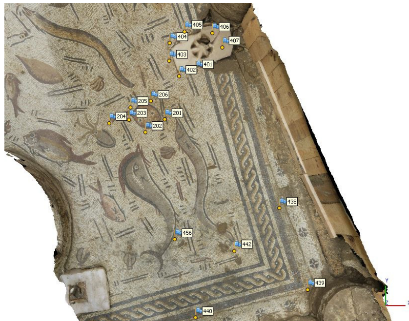
Figure 14. SfM model of the selected area with GCPs represented.
