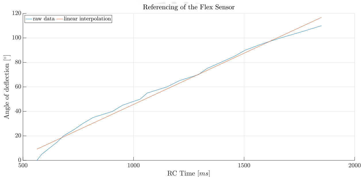
Figure 3.13: Calibration of the flex sensor with a RC-circuit
