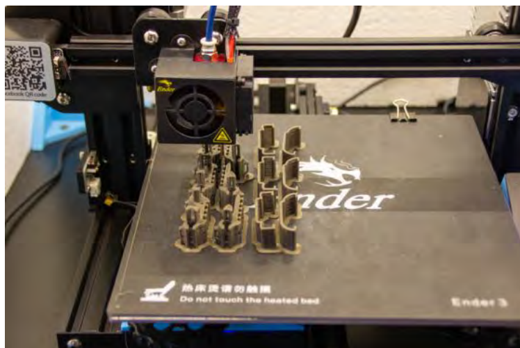
Figure 3.19: Fabrication of the Soft Robotic Gripper with a 3D-Printer
