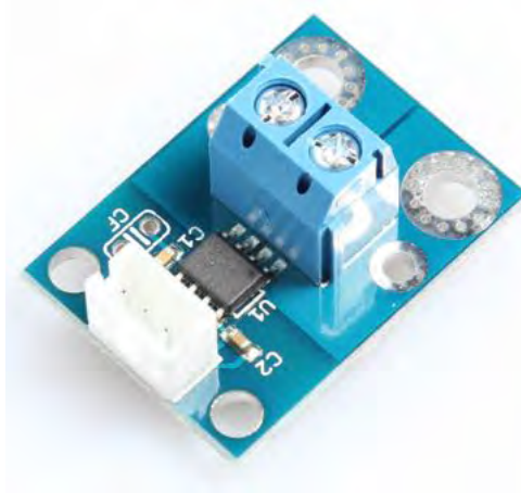
Figure 3.12: Linear current sensor from Microbot with an Allegro ® Hall-effect based IC, from [Mic20]
