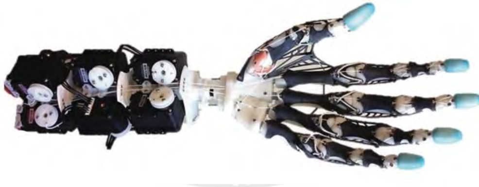
Figure 2.26: Biomimetic hand by Xu et al. Anthropomorphic design, driven by 10 servo motors [XT16]
