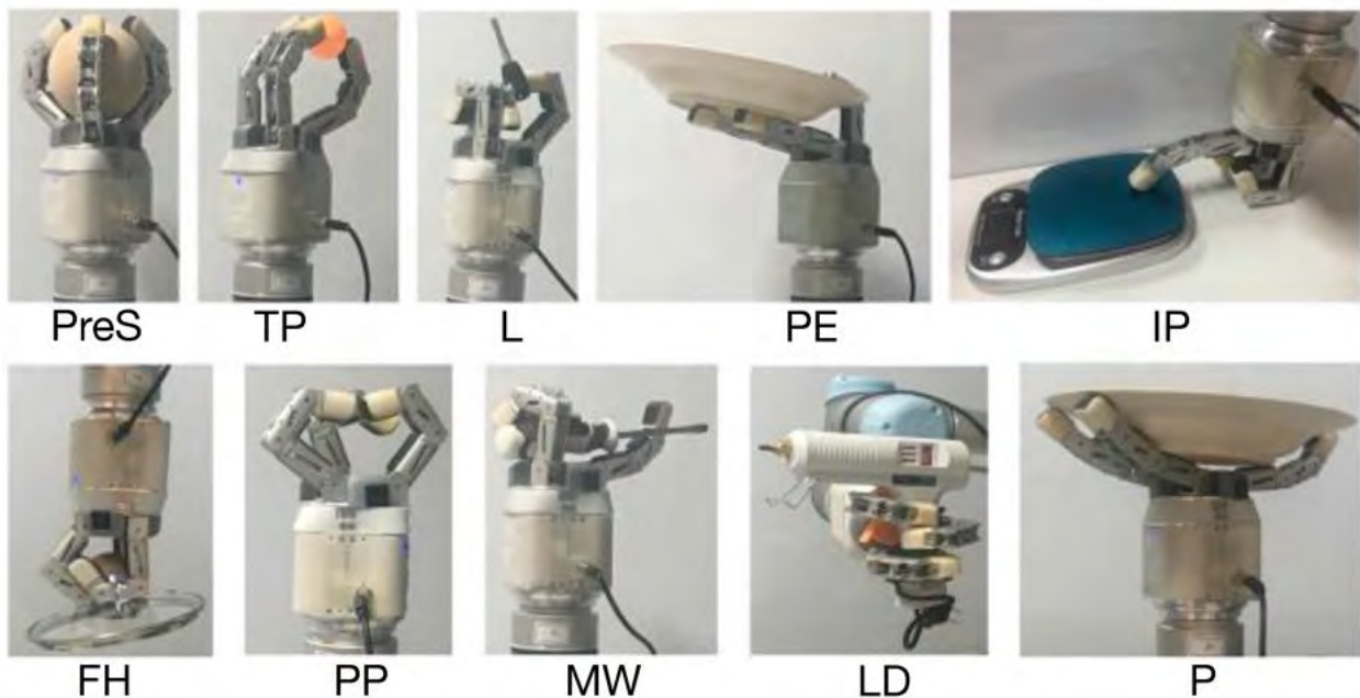
Figure 2.27: Grasping demonstration of the “Synergy-based Three-Fingered Hand” by Chen et al., integrated into the GRASP Taxonomy [Fei+16], modified from [Che+20] Precision Sphere (PreS); Tripod (TP); Lateral (L); Parallel Extension (PE); Fixed Hook (FH); Palmar Pinch (PP); Medium Wrap (MW); Large Diameter (LD). Two non-grasping postures: IP (index pointing/pressing); P (platform)
