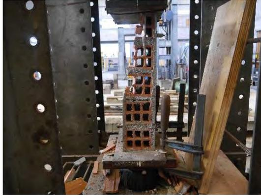
**Figura 6-5. Falla de Pila P-2.**
