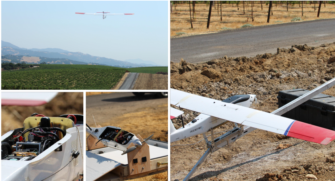
Fig. 4.3: AggieAir UAV capturing high-resolution imagery over the vineyard
