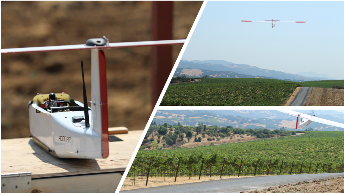
Fig. 3.2: AggieAir airframe layout flying and capturing imagery over the study area.
