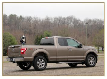
The portable Backpack system mounted on a carrier vehicle.
