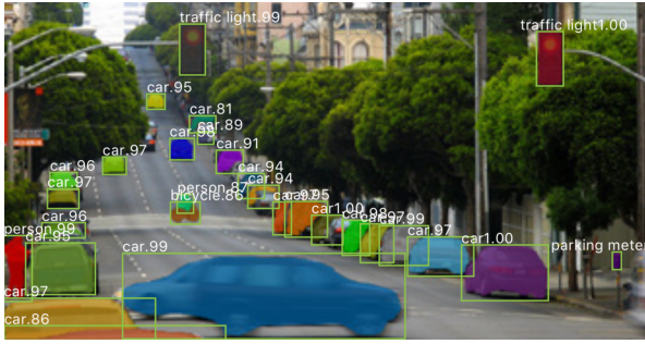
Figure 1: Sample Output of a Mask R-CNN Model. A Mask R-CNN model trained to recognize various types of objects in an image, including cars, traffic lights, parking meters, etc. The number next to each object label is the confidence of the class prediction. Image reproduced from [9].
