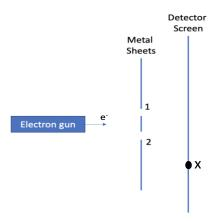
**Figure 4.** Double Slit Experiment with an electron gun
