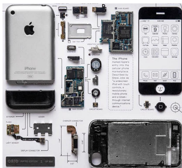
Figure 4. Hardware components of the first-generation iPhone, artwork by GRID ( https://gridstudio.cc ).
