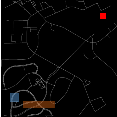
Figure 6. Grid environment with examples of sensor footprints of two types of scanning UAVs.
