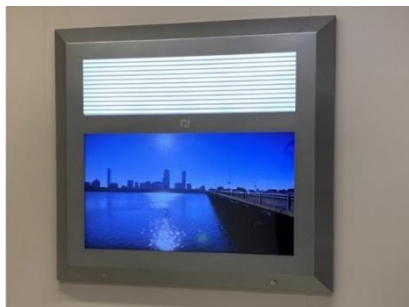
Figure 1. Virtual Window. A virtual window with a metal, tamper proof frame containing a natural light box and high-definition monitor (dimensions of virtual window frame 114cm x 127cm).
