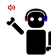
Fig. 2: Avatar responding to a tone stimulus in the right ear. Note, speaker icon is displayed to indicate to the technician that the tone was presented in the event the local speakers are not enabled.
