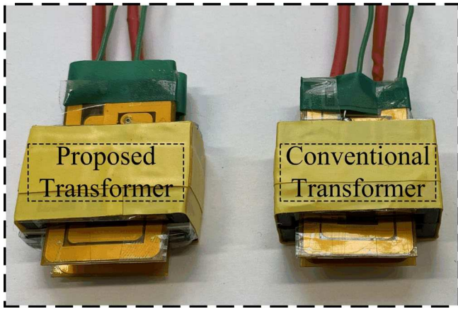
Fig. 9. Prototypes of the proposed and inserted-segmental-shunt (conventional) topologies. Core: E32/6/20/R-3F4.
