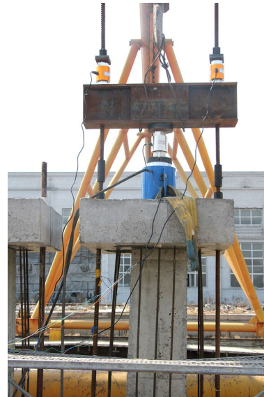
Figure 5. Test setup for prestressing reinforcing bars
