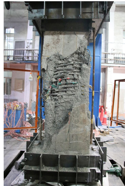
b) Local details of spiral stirrups
