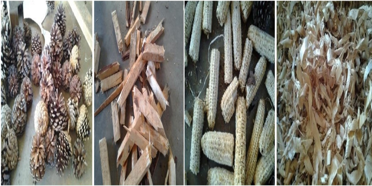
Figure 1. Study fuel types i.e. pine cones, wood pieces, maize cobs and wood shavings respectively
