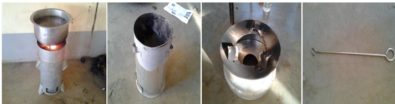
Figure 2. Gasifier stove, combustion/fuel chamber, concentrator lid and hook ended metal respectively
