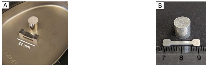
Figure 4-3: Representative compacts of compressive (immersion test) and microtensile test geometries of PM Mg-0.6Ca specimens. (A) After uni-axial hand pressing prior to sintering. (B) After sintering. The microtensile specimen shown in (B) is cut out from a thicker sintered part and, therefore, does not directly relate to the green part shown in (A).
