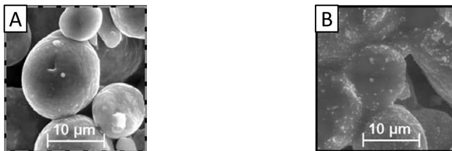
Figure 2-2: (A) Point contact between magnesium particles after sintering that are free from oxygen getter material. (B) Sinter neck formation between magnesium particles when surrounded by oxygen getter material [32]. With permissions to reprint from WILEY-VCH Verlag GmbH.
