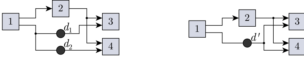
(a) Hyperedge with two dummy nodes (b) Hyperedge with one dummy node
