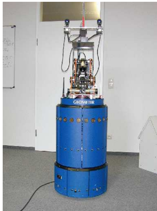
Fig. 6.1: The B21 experimental mobile robot. The robot is equipped with 24 sonar, 56 infra-red, 32 tactile sensors, and a binocular CCD camera.
