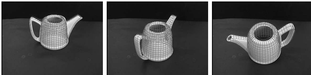
Fig. 4.2: First pose results of the tea pot. The projected object model visualizes the quality of the 3D pose.
