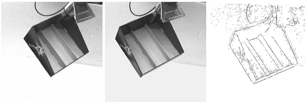
Fig. 6.11: Example for 3D reconstruction from stereo. From left to right: image from left camera, image from right camera, and representation of corresponding line segments which have been found.
