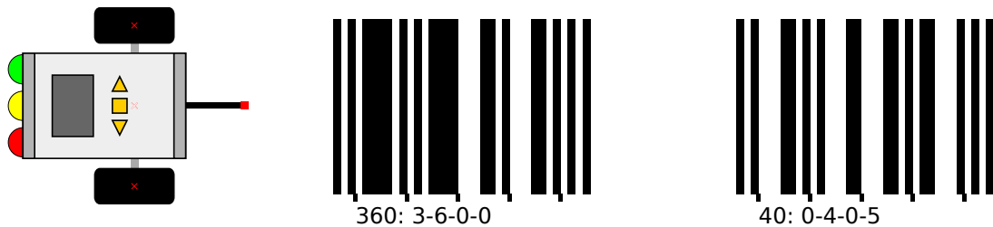
Figure 2.5.: An example how the SVG for simulating the barcode reader looks like. The corresponding JavaScript also allows the visualization to work as an environment by setting input variables for the controller in form of the light value.
