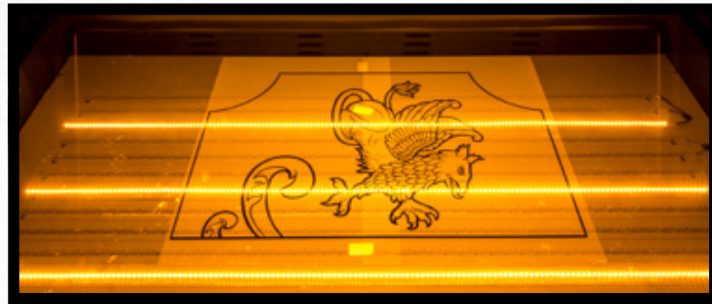
FIG. 3.30 | FIG. 3.31 | Inkjet-printed transparency lying on UV machine | Photos by the author
