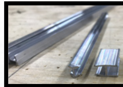
FIG. 3.2 | Lead came, showing the “H”-shaped cross-section that allows glass pieces to be conjoined | Photo by the author
