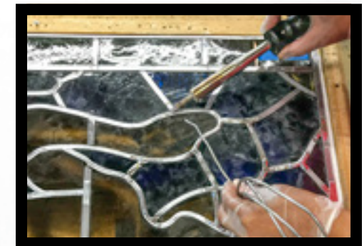
FIG. 3.3 | A glazier soldering lead strips together around painted glass pieces | Photo by the author
