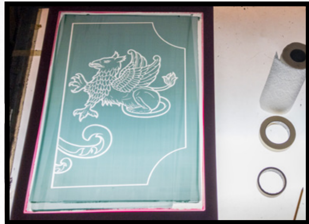
FIG. 3.32 | A finished screen, ready for printing onto a piece of glass | Photo by the author
