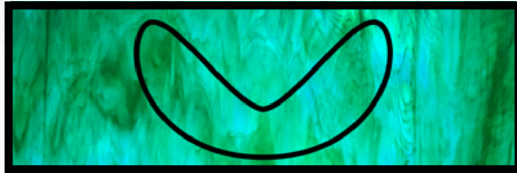
FIG. 3.4 | A shape that is structurally unsound, due to the weak point created by the sharp inward curve | Photo by the author
