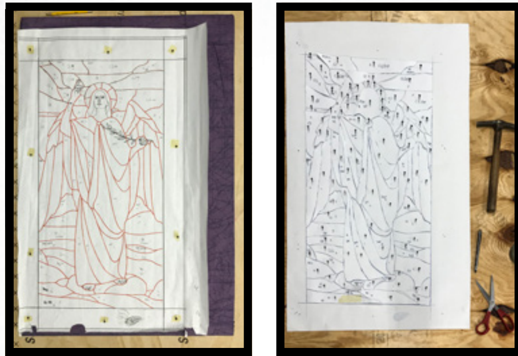
FIG. 3.8 | FIG. 3.9 | The traditional, carbon-copy process for creating cutlines and patterns | Photos by the author
