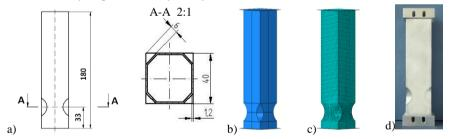
Fig. 1. Column models: a) general view, b) geometrical model in Abaqus FEM system, c) FE model, d) specimen A30 installed in blocs with vents
