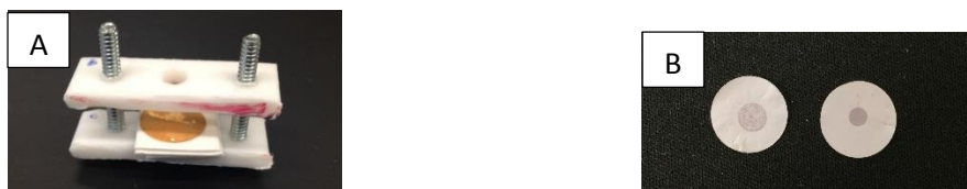
Figure 20. (A) A home-built blotting apparatus: four sheets of blot paper were layered on the Teflon base and the membrane was placed on top. A rubber O-ring (4-mm inner diameter) was placed between the membrane and top Teflon sheet. (B) the size comparison of two spots of aggregates obtained after filtration via the home-built blotting apparatus (left) and 48-well Bio Dot blotting apparatus (right). Each filter diameter is 13 mm.
