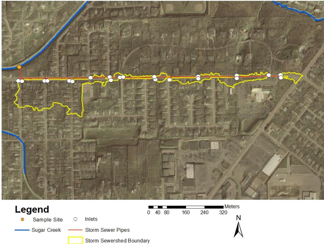
Figure 4. A Long and Skinny Storm Sewershed. This storm sewer system follows a single road, the storm sewershed reflects this shape.
