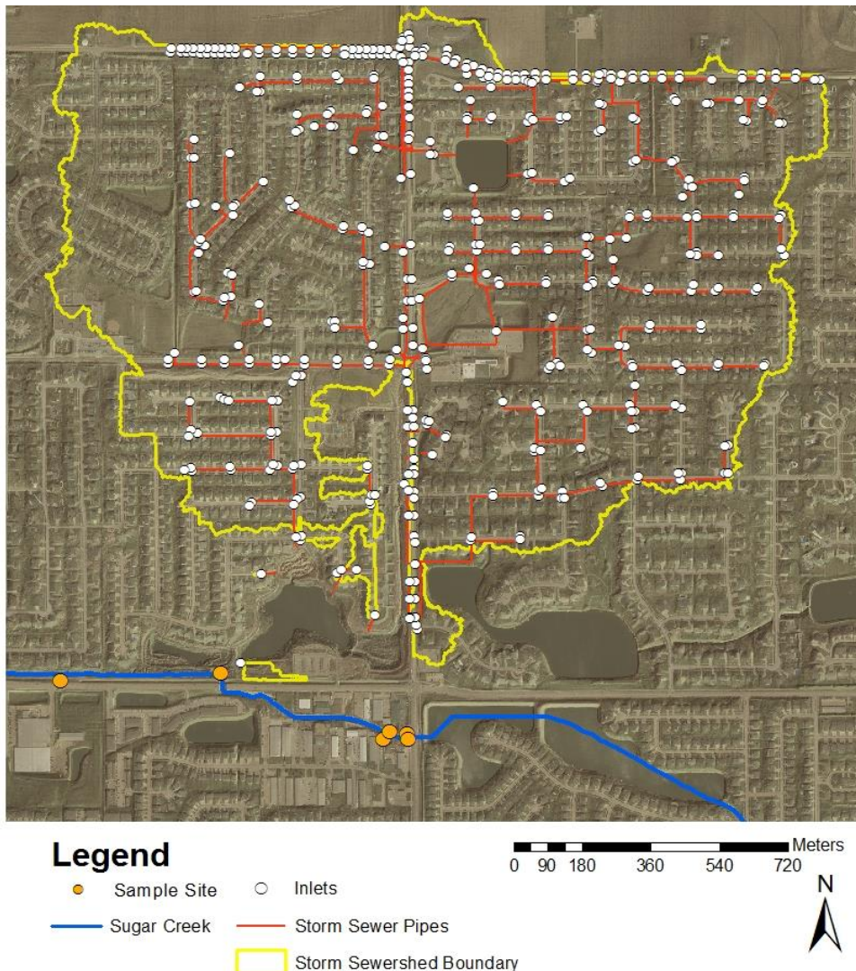
Figure 5. A Square Storm Sewershed. This storm sewer system has many branches. The contributing area generally creates a square-like polygon around it.
