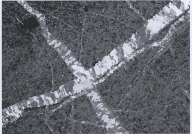
Figure 7. Tensional stress preserved in two generations of quartz veins (gypsum plate). Note the fibrous habit of quartz grains in veins.
