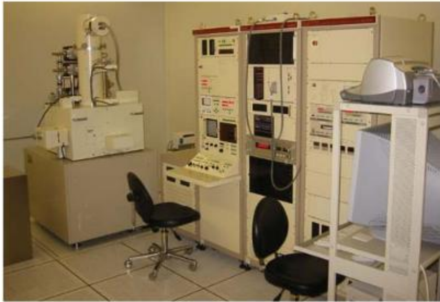
Fig. 3-11 Elionix 7700 75kV e-beam lithography system.
