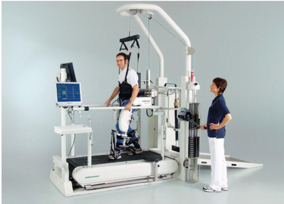
Figure 1-3. Robot-aided gait rehabilitation training with a therapist supervising the training session. (reprinted from http://ptjournal.apta.org/content/85/1/52/F1.large.jpg ).
