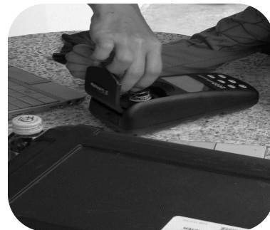
Water sample measurement using a portable turbidity meter
