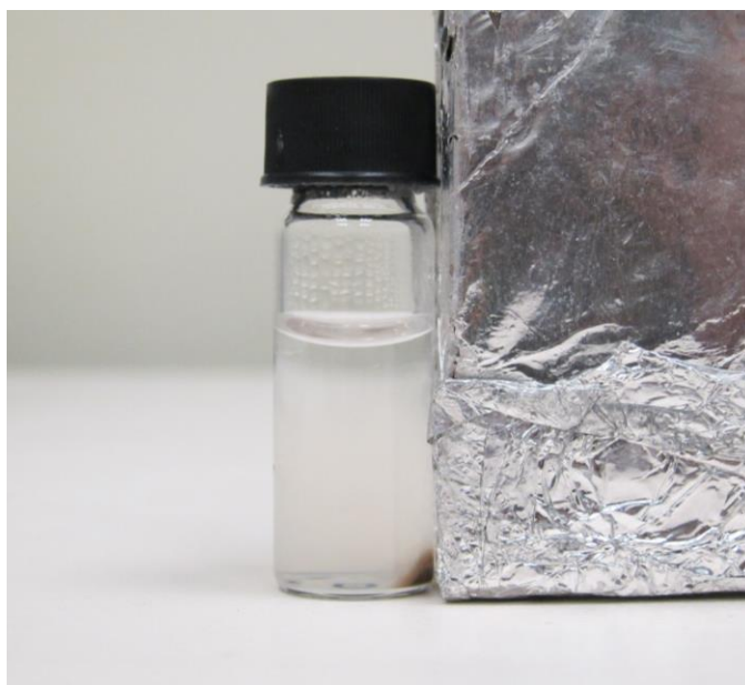
Aqueous suspension of Gd-doped manganese silicate separated from the solution through magnetism
