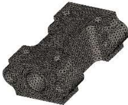
Figure 5-21: Mesh model of the centre casing
