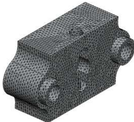
Figure 5-12: Mesh model of the inner cover
