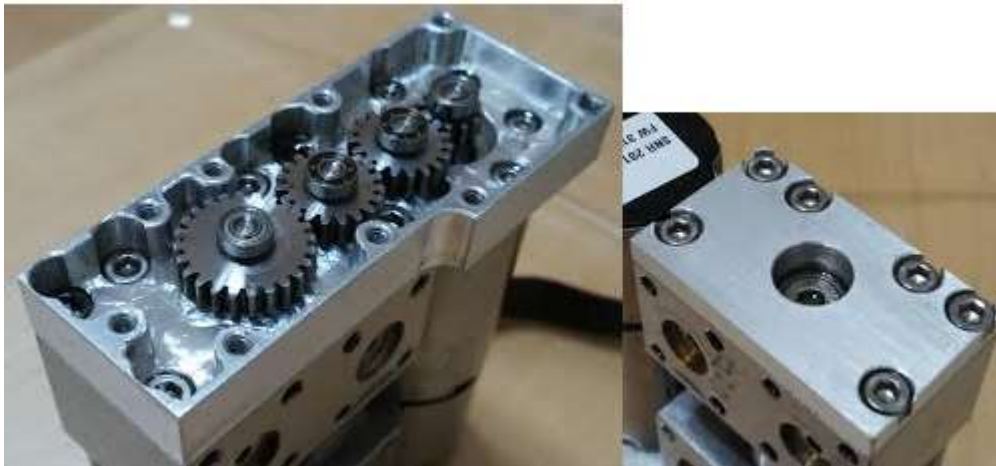
Figure 4-1: Input forward base housing the gear train (left) and aft base (right)
