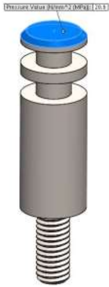
Figure 5-7: Load on model of input piston
