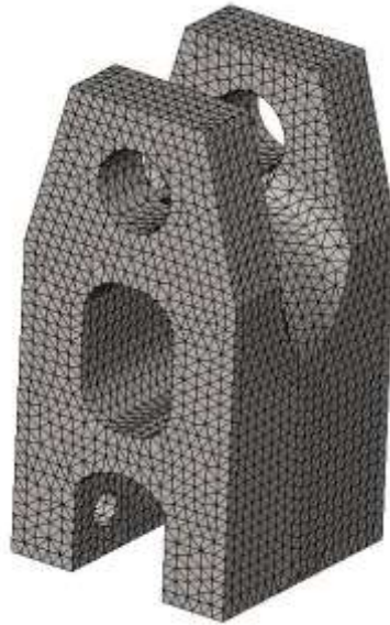
Figure 5-30: Mesh model of lever arm
