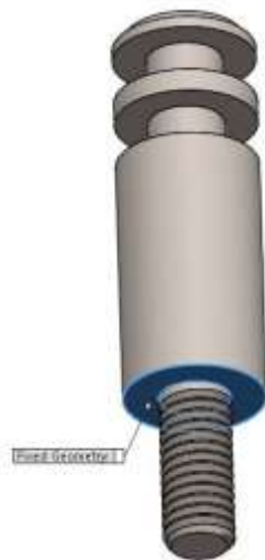
Figure 5-6: Constraint on model of input piston
