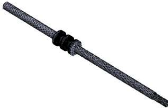
Figure 5-26: Mesh model of output piston
