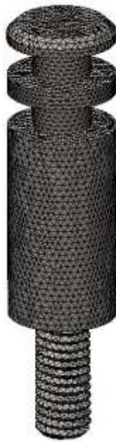
Figure 5-8: Mesh model of input piston
