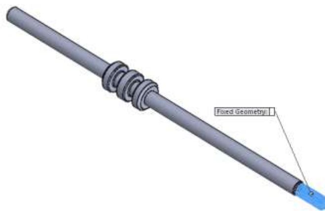
Figure 5-24: Constraints on model of output piston
