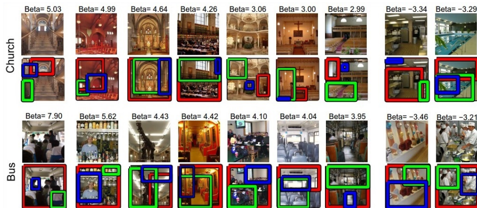
FIGURE 2.2: Prototypes for two Indoor67 categories ( church_inside and inside_bus ), sorted by their weights. First 7 columns correspond to highest ranked, while last 2 columns the least ranked prototypes for shown category. Thickness of ROI's bounding box is proportional to its weight. Adopted from [106].
