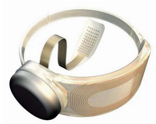
Figure 1.1 Retinal implant with wireless interface [10]
