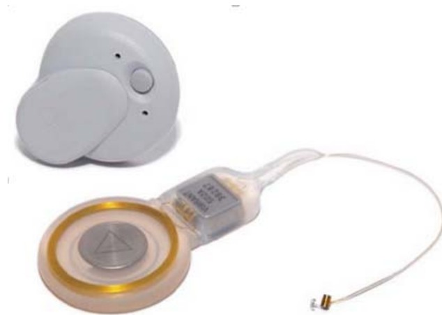
Figure 1.2 Middle ear implantable device powered via inductive couple coils [15]
