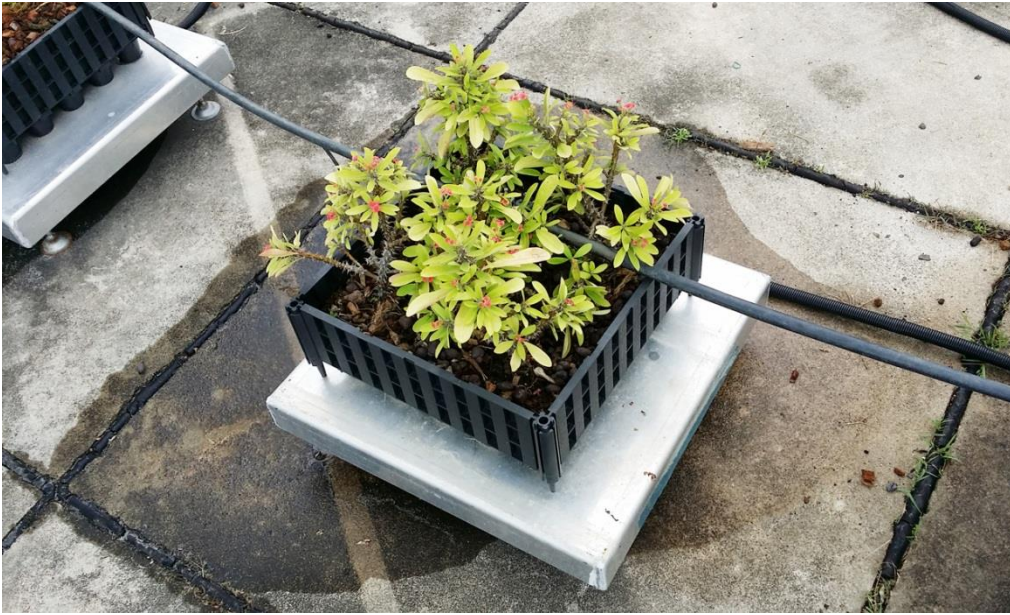
Figure 81. Rooftop greenery panel on load cell
