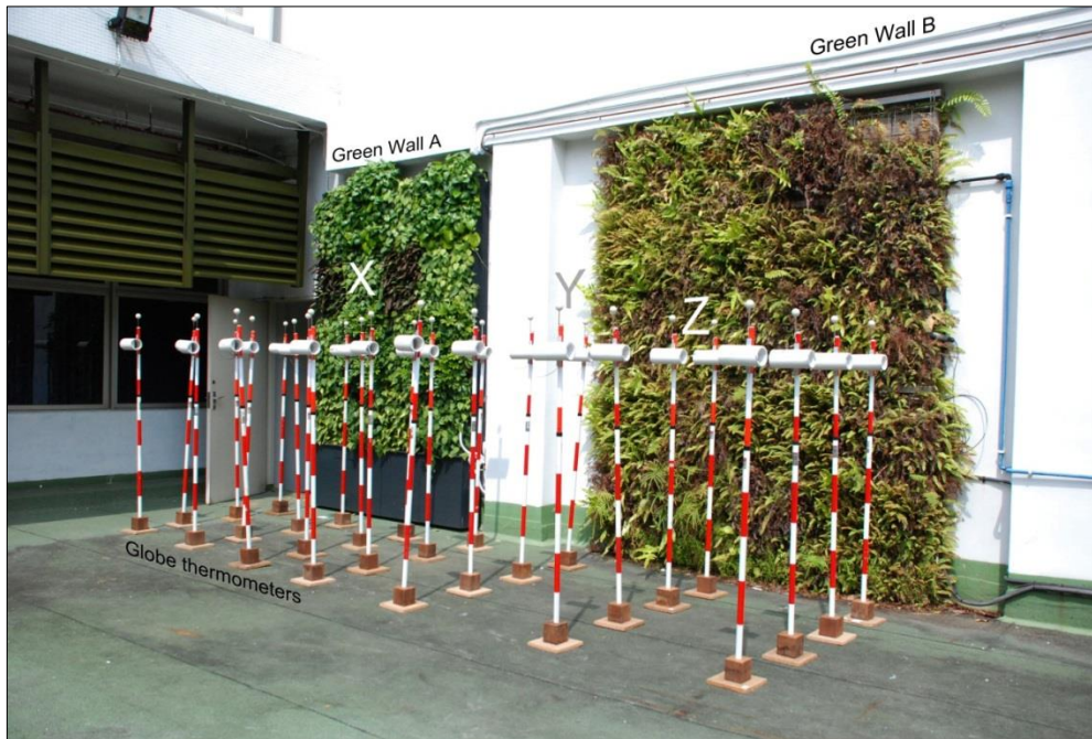
Figure 107. Measurement setup. Globe thermometers were attached to poles with white PVC pipes housing surface and air temperature loggers.
