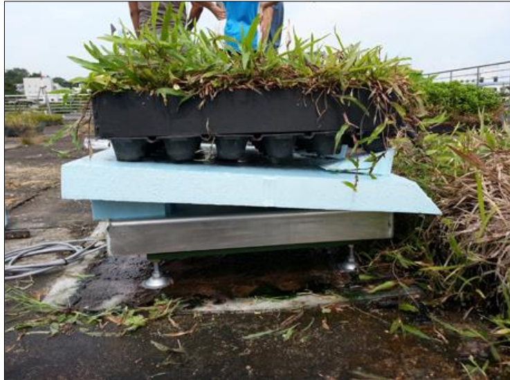
Figure 30. Measurement of plant evapotranspiration rate with load cell
