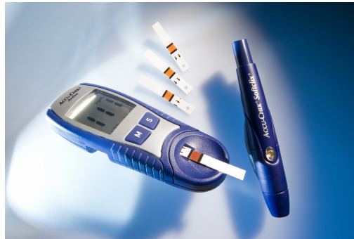
Figure 1.2: Capillary blood glucose monitor (Roche Accu-chek Active) with disposable sensor strips and fingerprick device holding lancets.
