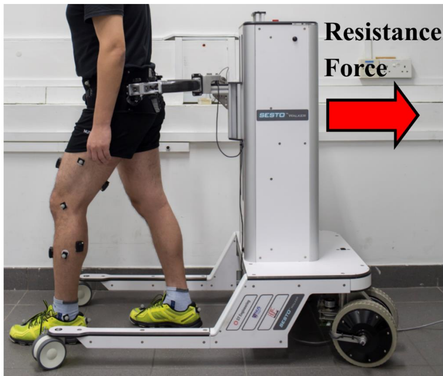
Fig.VI-1 The robotic walker and anterior force applied with increasing resistance
