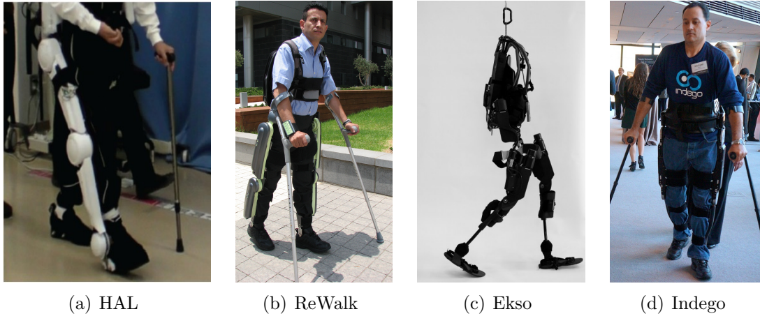
Figure 2.3: Overground wearable gait trainers (HAL, ReWalk, Ekso, Indego)
