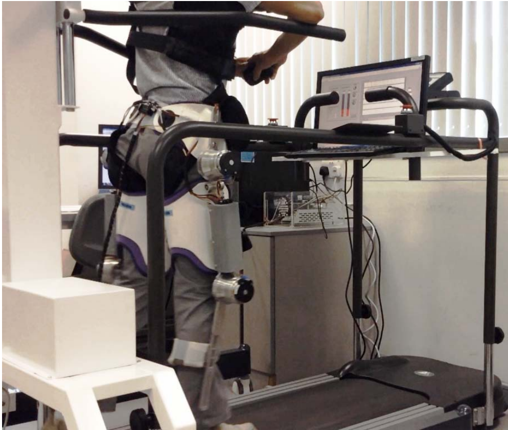
Figure 5.4: The experimental setup: the subject was wearing the assistive device and performing treadmill gait training with body weight support
