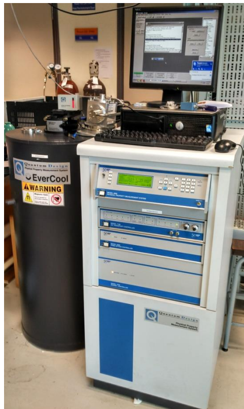
Figure 3.18 A photograph of our PPMS system mainly for electrical properties measurements.
