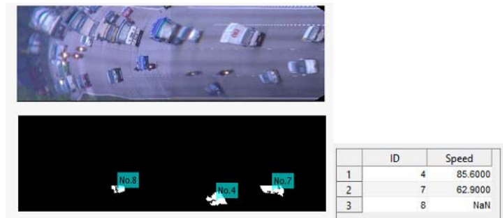
Figure 6.11: An example of the speed calculation step (km/hr).
