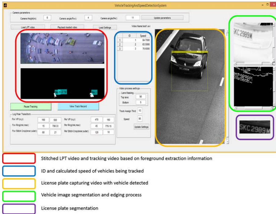
Figure 6.17: Results of the composite vision system integrated with the license plate detection module.
