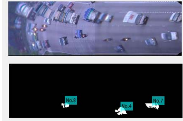
Figure 6.8: Vehicle tracking with Kalman filter.
