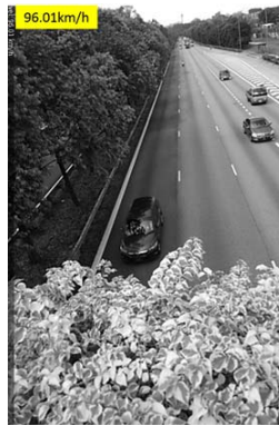
(c) Sample output of the Speed Radar Cam application. Top left shows the speed of the nearest vehicle.
