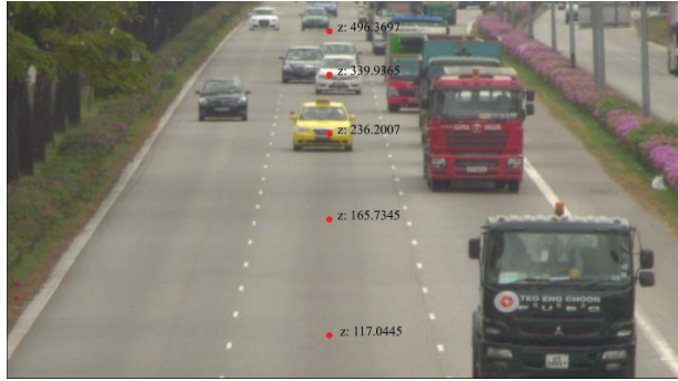
(a) Verification using separation of the lane markers.
