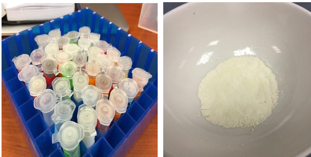
Figure 2-4 Synthesized \text{Bi}_2\text{O}_3/\text{TiO}_2 heterojunction nanocomposites.
