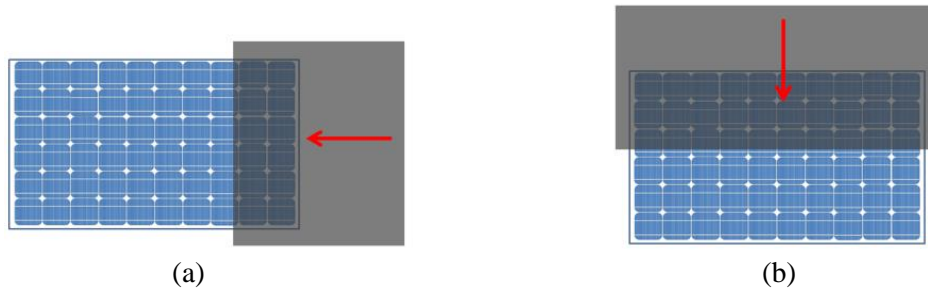
Figure 6.4: (a) The shadow moves horizontally; (b) the shadow moves vertically.
