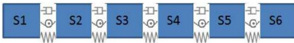
Fig. 2.3 Topological relationship of linear-elastic representation in soft body simulation [1].
