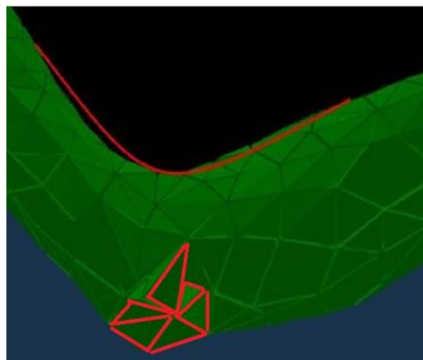
Fig. 4.8 Simulation of aortic rupture when a part of the meshed model was detached from the aorta
