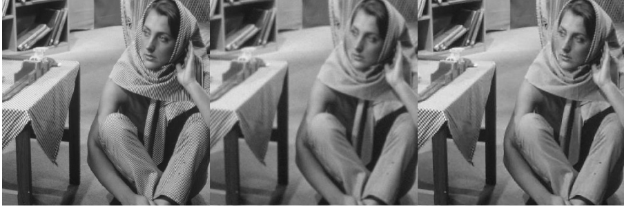
FIGURE 1.2.1. Deblurring results for the test image “barbara”. Columns 1 to 3 contain respectively the original image, blurred image and deblurred image.
