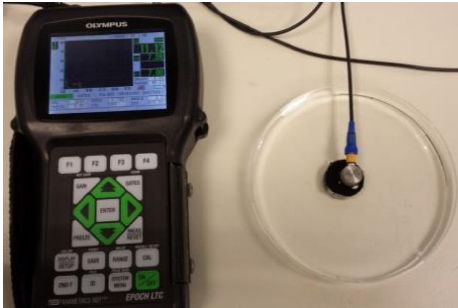
Figure 3.4: 2.25MHz transducer placed on top of submerged composite sample. RF waveform readings can be collected from the Epoch LTC Handheld Flaw Detector device.
