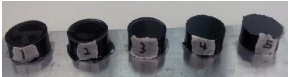
Figure 3.3: Cylindrical samples of CNF/CNT-PDMS nanocomposites with varying mass fraction of fibers after curing.
