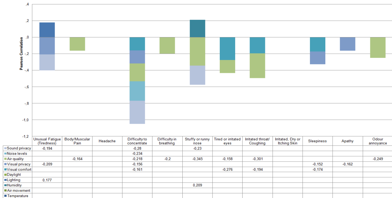
Figure 48 – Correlations between building related health symptoms and IEQ perceptions in GM buildings
