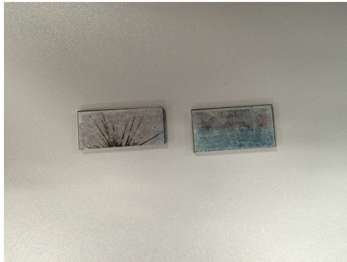
Figure 4.15: Examples of sample with expulsion and sample without expulsion.
