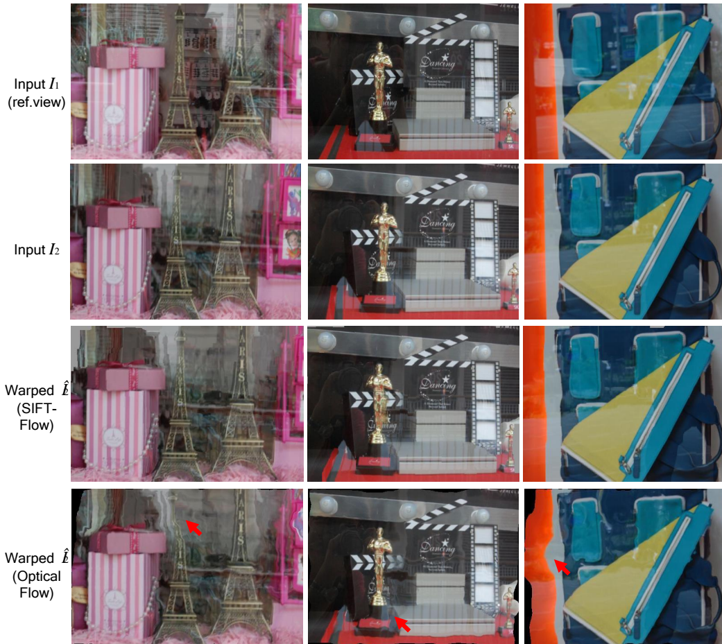
Figure 3.3: We have compared optical flow with SIFT flow in aligning the input set. For the optical flow, we used the popular Classic+NL method [Sun et al. 2014].
