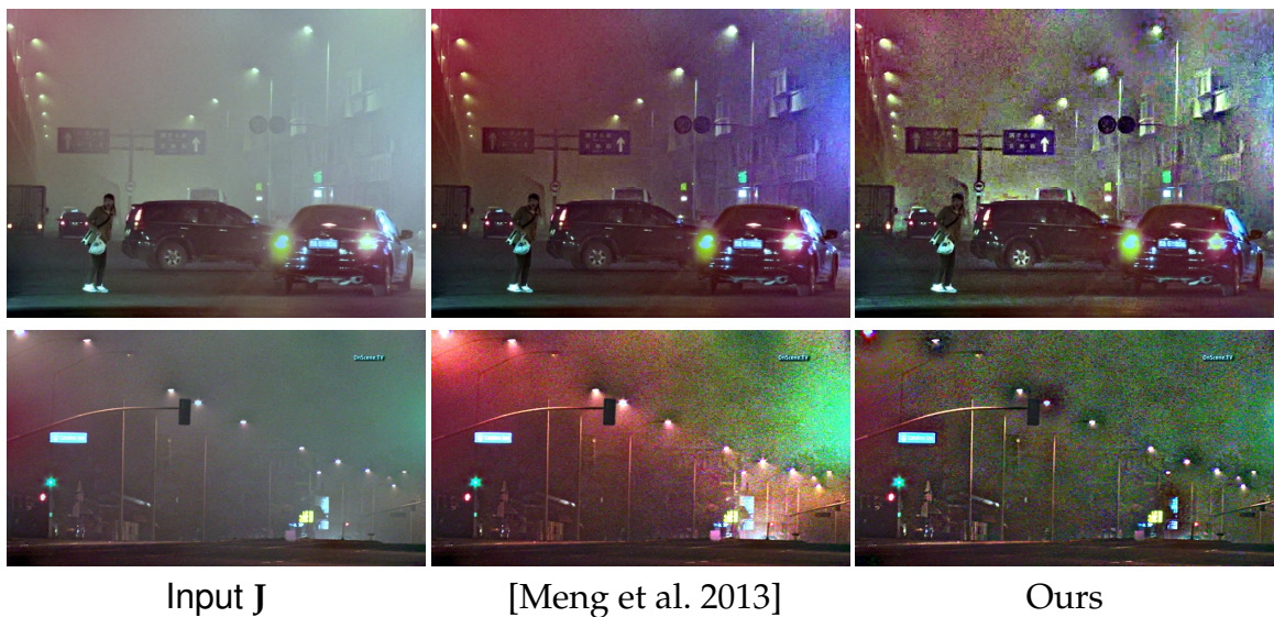
Figure 5.7: The left column shows the haze images, J , after decomposing it from the glow images. The middle column shows the dehazing results using an existing daytime dehazing method [Meng et al. 2013]. The colors are noticeably shifted due to the varying atmospheric light. Right column shows our results, where the color shift is less significant since varying atmospheric light is used.
