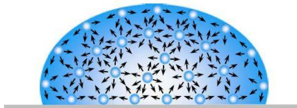
Figure 1.1.1 Schematic explaining the origin of surface tension in liquids.[6]
